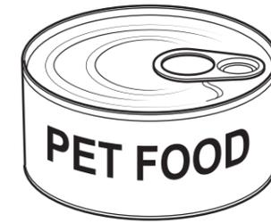
Complete the drawing of the tin of pet food below by adding the top ellipse and bottom half ellipse. Major axis 90 mm. Minor axis 30 mm. The two sides of the tin are given. [7]
