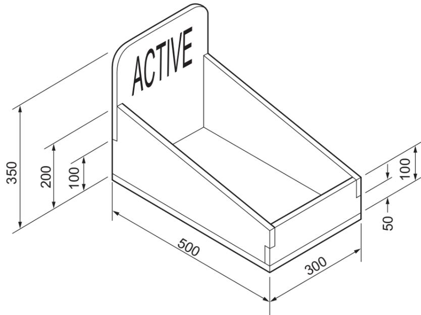
(a) Complete the parts list by drawing the pieces of the point of sale display to a scale of 1:10. [12]
