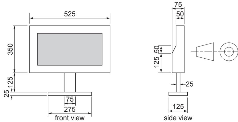
(a) Complete the 60/30 planometric view of the flat screen television to a scale of 1:5 in the space below. [10]
