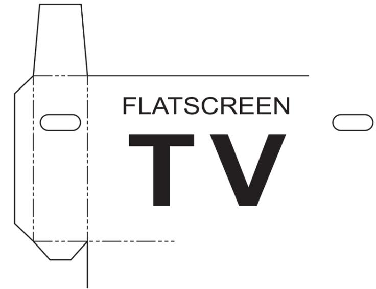
(i) Complete the development (net) of the package for the flat screen television to a scale of 1:10. [10]
