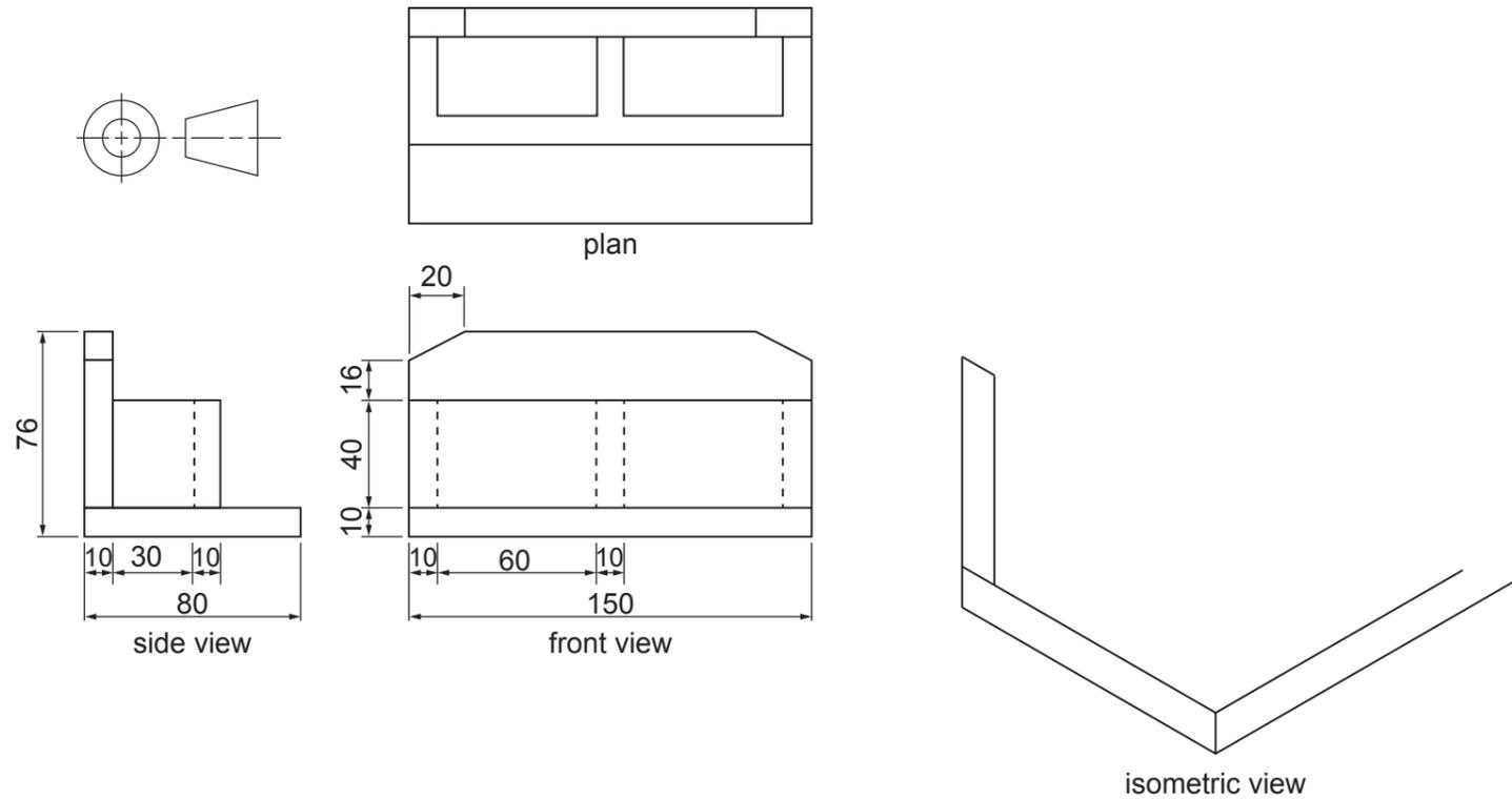
(a) Complete the isometric view of the remote control holder to a scale of 1:2. [13]
