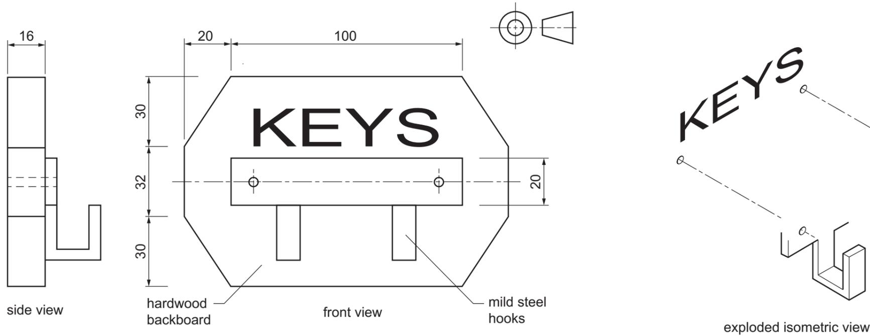
(a) Complete the exploded isometric view of the key rack to a scale of 1:2. [12]
