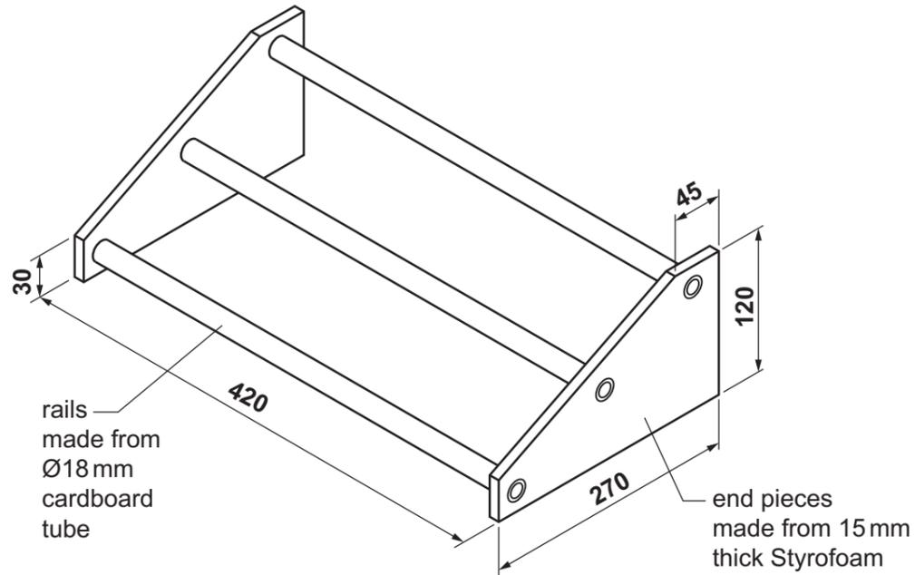
(a) Complete the orthographic views of the shoe rack below to a scale of 1:3 by adding:
