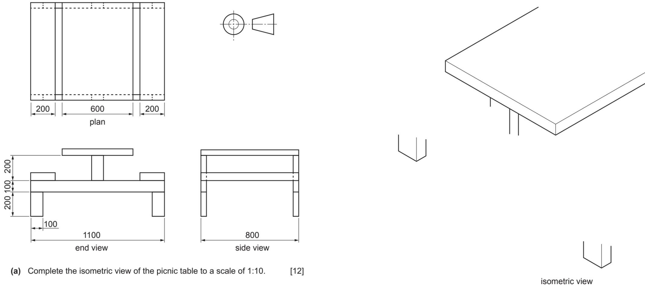
(a) Complete the isometric view of the picnic table to a scale of 1:10. [12]
