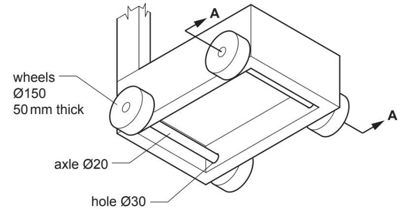
Complete the sectional view **A-A** through the axle of the toy trolley to a scale of 1:5. [6]
