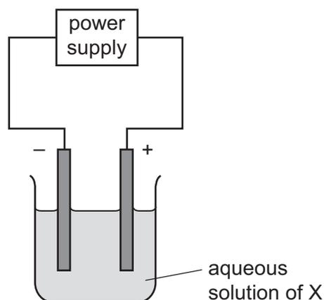
Hydrogen is produced at the cathode and chlorine is produced at the anode.
