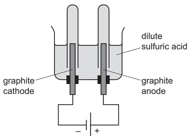
$30\text{ cm}^3$  of a gas is collected at the cathode. A different gas is collected at the anode.
